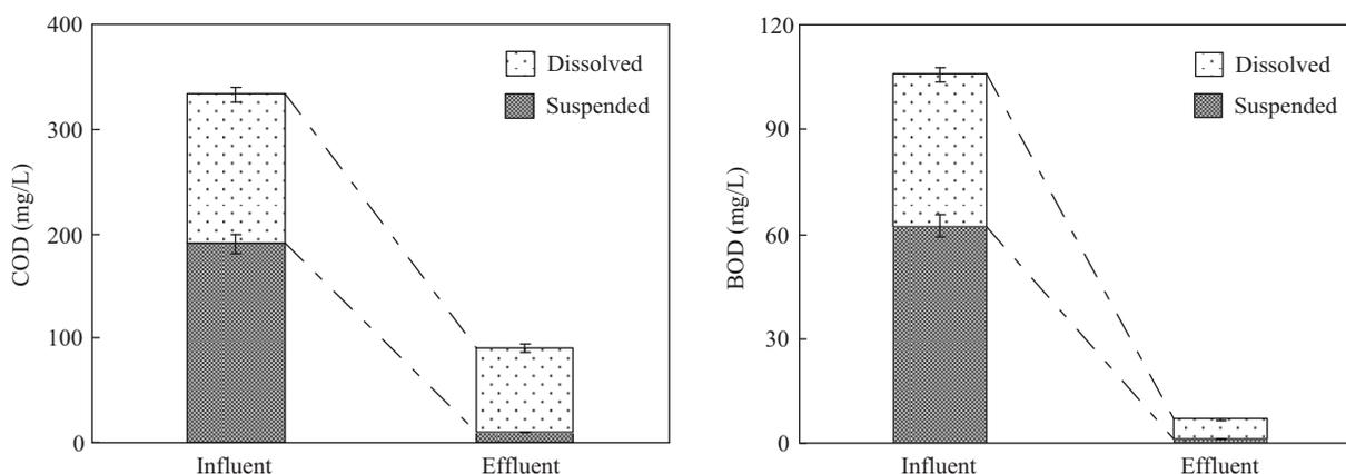
Fig. 6 Distribution and removal of dissolved and suspended COD and BOD by the CWs.
