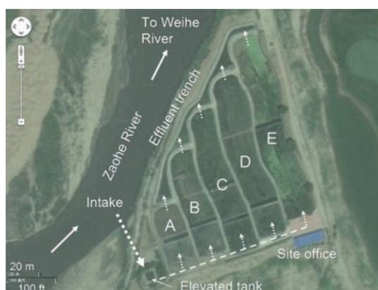
Fig. 2 Satellite view of the pilot constructed wetlands (CWs) and the flow diagram.
