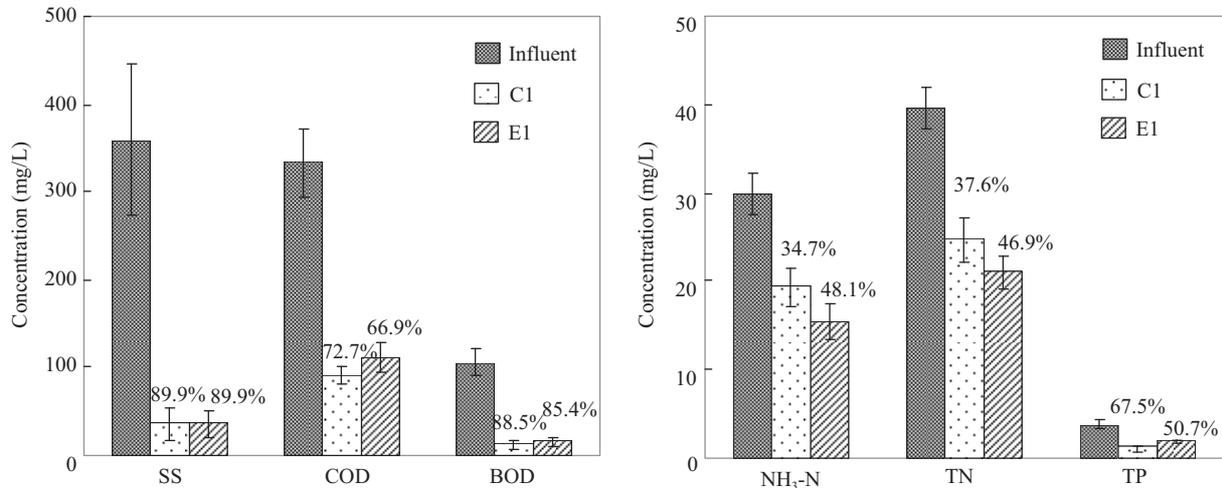
Fig. 3 Comparison of pollutants removal by SSF (C1) and FWS (E1) cells under similar operational conditions.
