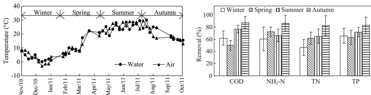
Fig. 7 Seasonal variation of air and water temperature and pollutants removal by System E throughout the experimental period.
