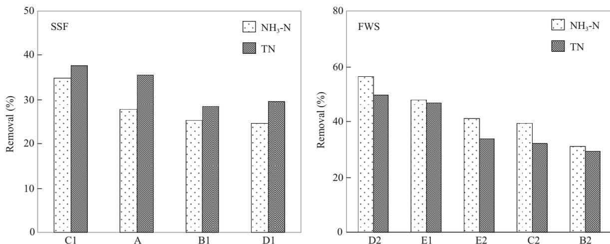
Fig. 4 Comparison of NH<sub>3</sub>-N and TN removals by SSF and FWS cells.
