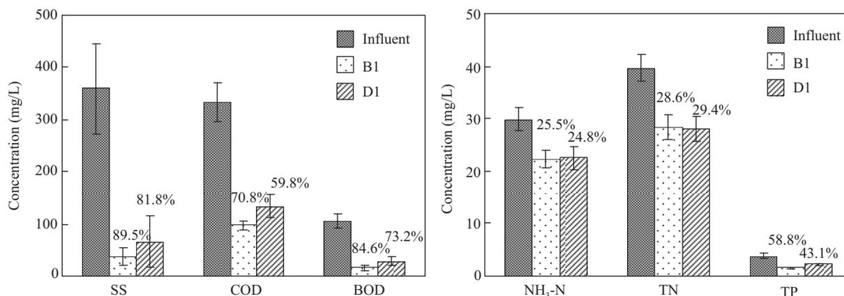
Fig. 5 Comparison of pollutants removal by SSF cells with slag (B1) and gravel (D1) as substrates under similar operational conditions.
