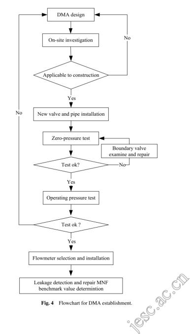
and lessons learned from the pilot schemes (Fig. 4). These approaches normally consist of a series of sequential steps such as: on-site investigation, new valve and pipe installation, zero-pressure test, operating pressure test, flow-meter selection and installation, leakage detection and reparation, and the determination of a benchmark value for the minimum night (Xu et al., 2008).
