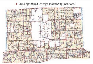
Fig. 2 Optimized leakage meters distribution plan within the 2nd ring belt of Beijing.
