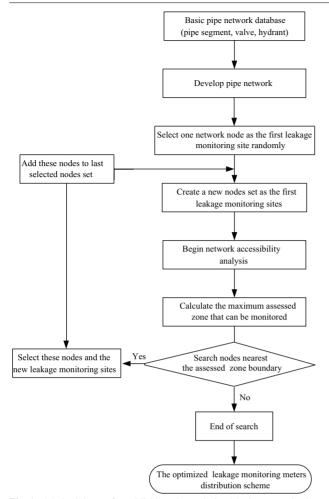
Fig. 1 Methodology of establishing the optimized leakage monitoring meters distribution scheme
