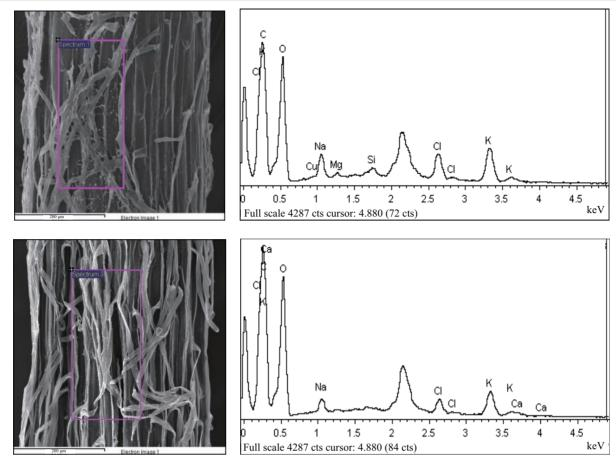
Fig. 6 SEM image and EDS of wheat root surface after exposure to 200 mg/L CuO-NPs (above) and then washed with 10 mmol/L Na<sub>4</sub>EDTA and ultrasonic (bottom).
