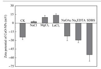
Fig. 3 Effect of washing reagents (10 mmol/L, pH 6.0) on zeta potential of CuO-NPs.
