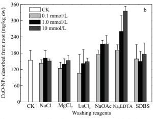
Washing reagents Washing reagents on desorbing CuO-NPs from wheat root after pre-exposure to 20 mg/L (a) and 200 mg/L (b) of CuO-NPs. dw: dry weight.
