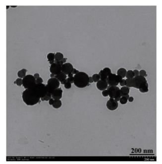
Fig. 1 TEM image of CuO nanoparticles
