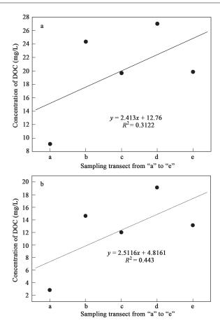
Fig. 4 A fit map of horizontal variations of DOC in annular wetland soilwater solutions from "a" to "e". (a) horizontal variations of DOC in soil pore water at depth of 10–20 cm; (b) horizontal variations of DOC in soil pore water at depth of 20–40 cm.
