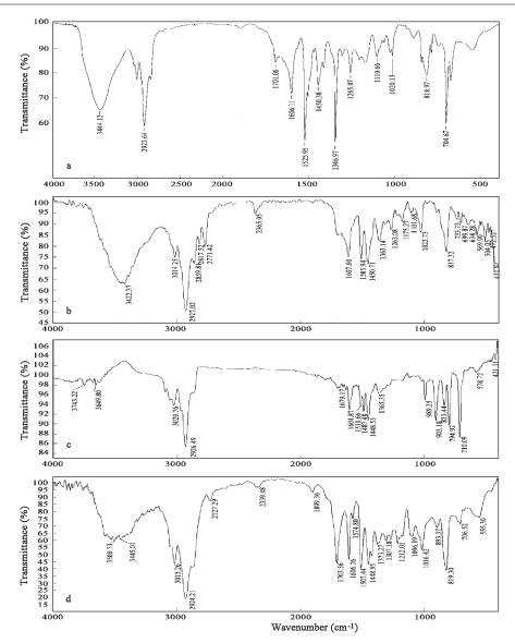
Fig. 1 IR spectra of the polymeric adsorbents. (a) NG-10; (b) NJ-99; (c) XAD-4; (d) CHA-111.
