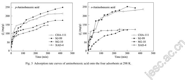
Fig. 3 Adsorption rate curves of aminobenzoic acid onto the four adsorbents at 298 K.
