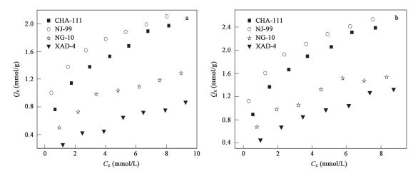
Fig. 2 Adsorption isotherms of aminobenzoic acid on different adsorbents (298 K). (a) p-aminobenzoic acid; (b) o-aminobenzoic acid.
